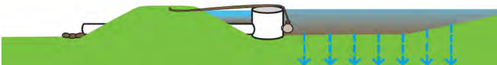
Figure 5D Sediment particles start to settle and pond water infiltrates into the underlying soil.
