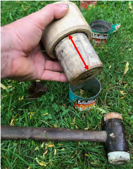
2b Option – drive in with a mandrill.
