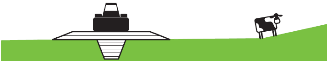
Figure 21 Compact fill in thin 150 mm–200 mm layers using a dedicated Roller.
