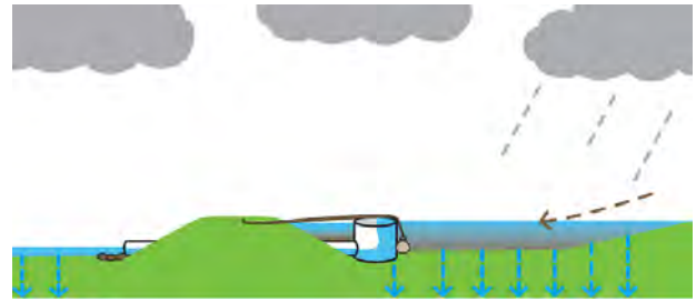
Figure 3.2 Storm water run-off capture and infiltration.
