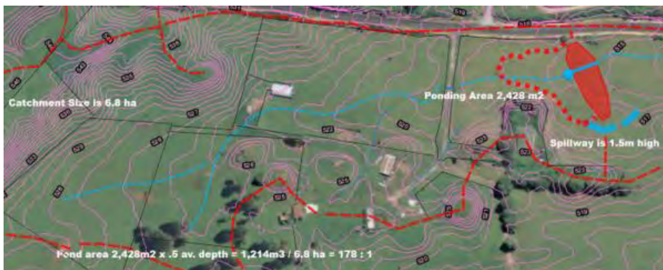
Figure 2 A typical DB 'mock-up' with ponding volume and catchment size drawn by use of GIS with LiDAR data. Here the storage to catchment area ratio is 178:1.
